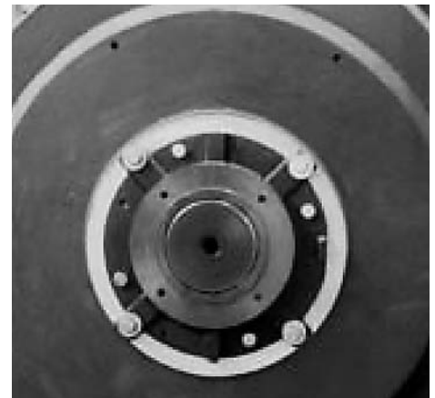
Accessory Face for mounting tachometer. Typical construction for Frame GK280.
