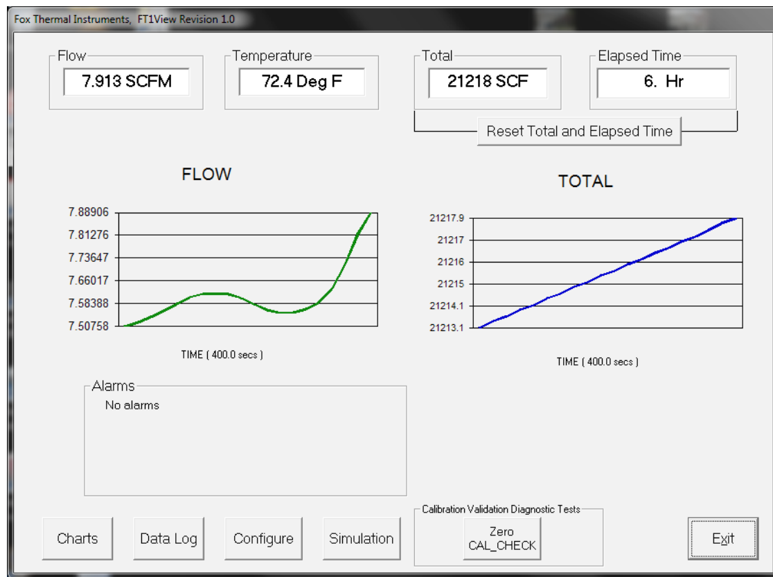
Fig. 3.1: FT1 View™ Main Screen
