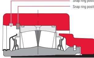
Snap ring position for expansion Snap ring position for non-expansion
