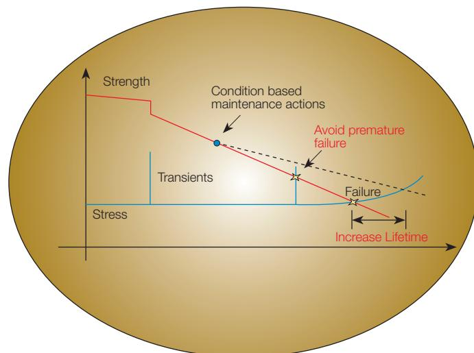
*"Insulation material in electrical machines is exposed to thermal, electrical, mechanical and environmental stresses during operation. Over time these stresses cause aging of the insulation material. Aging is represented by the red curve. Stresses from normal operation and abnormal events (such as transients) are represented by the blue curve. When the blue and red curves cross, an insulation failure will occur leading to expensive unplanned downtime."*
