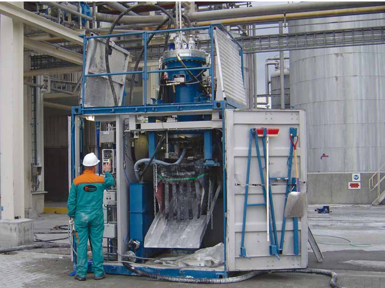
The Booster range is a compact design and easy to install, as shown here in a container to allow mobile and temporary production.
