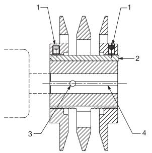
NOTE: Key (2) protrudes to provide a better grip when removing.
