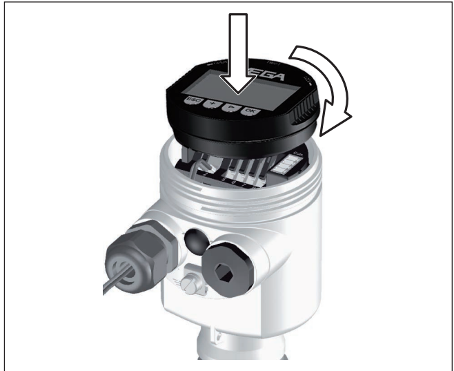
Fig. 27: Insert display and adjustment module in the single chamber housing
