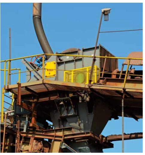
The Toledo Docks facility has run more than 3 million tons of ore since the installation of the Baldor Dodge Hydraulic ISAF (located behind the yellow guard) on its new high-flow shoot. Because of the bearing's reliability, ease of installation and expected ease of removal, company officials expect more Hydraulic ISAF units will be installed in the future.
