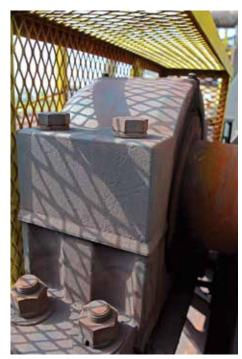
Baldor's Dodge Hydraulic ISAF pillow block bearing, with its patented, integral hydraulically assisted mount and dismount system, is quick and easy to install and remove. A built-in hydraulic piston is used on both the mount and dismount nut to facilitate tightening the bearing on the shaft during installation, and then aid in removal when it is time to dismount and replace the bearing. A harsh-duty, two-part sealing system protects the bearing from contamination and extends service
