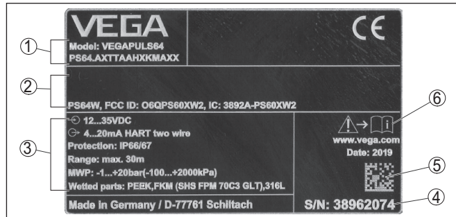
Fig. 1: Layout of the type label (example)
