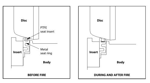
Wafer-Sphere butterfly valves with Fire-Tite seats have been tested and approved to API 607 Edition 4 and to BS6755 part 2.
