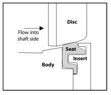
When pressure is on the non-insert side, the disc moves into the seat. Due to the spherical profile of the disc, the more the disc moves into the seat, the tighter the shut-off. Excessive movement of the seat is limited by the flexible lip which contacts the bottom of the groove in the insert ring.
