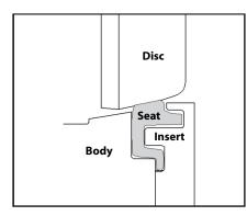
When the valve is shut, the disc slightly deflects the seat. This slight deflection "energizes" the seat. While energized, the sealing surface of the seat is constantly pushing against the edge of the disc.
