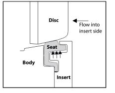
When pressure is on the insert side, pressure is applied under the seat lip. This further amplifies the sealing force between the disc and the seat.
