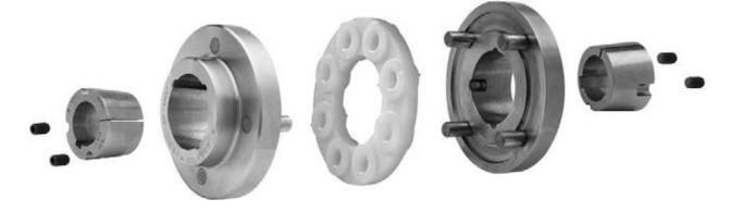
POLY-DISC flexible couplings use a non-metallic disc molded of a polyurethane compound to transmit torque. A special heat treatment after molding, refines the physical properties of the disc that allow it to remain pliable to cushion shock loads and still have resistance to most common chemicals such as acids, alkalis and petroleum products. The disc has an operating temperature range of -90° F to +170° F.
