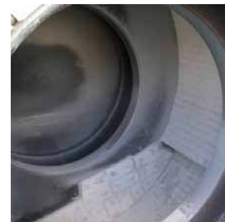
Ceramic linings give outstanding wear life
